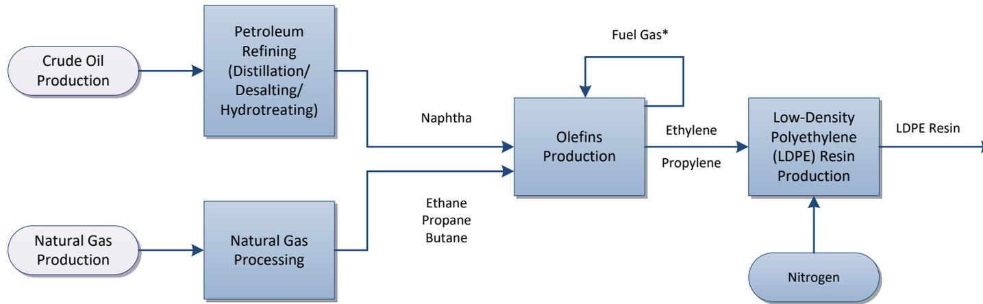
**Figure 2. Flow diagram for the Production of Low-Density Polyethylene (LDPE).**
