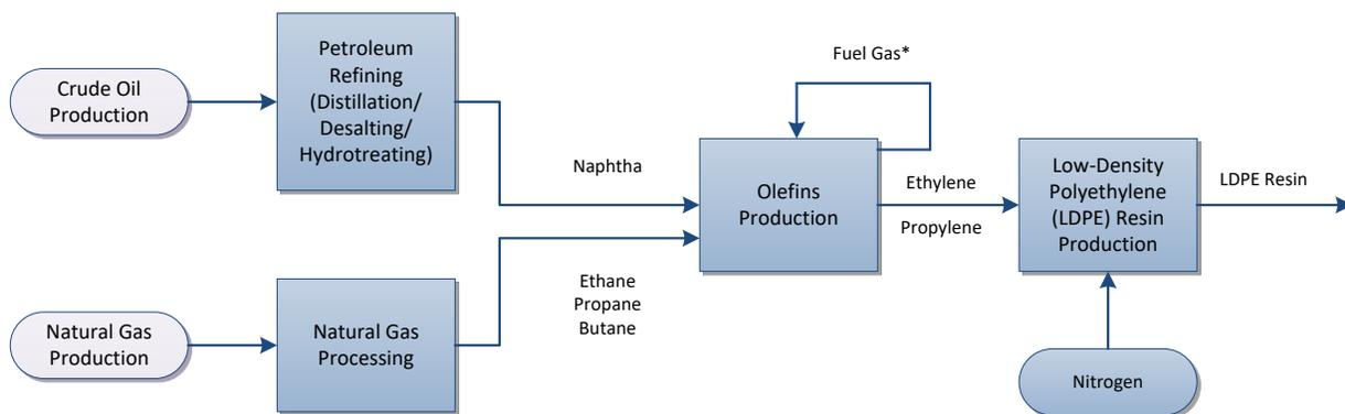
**Figure 15. Flow diagram for the Production of Low-Density Polyethylene (LDPE).**
