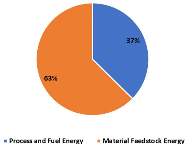
**Figure 3. Process/Fuel and Material Feedstock Percentages for LDPE Resin**
